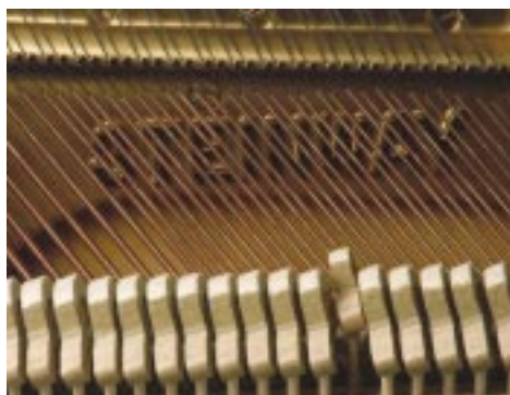
Figure 3 The strings and hammers inside a piano
